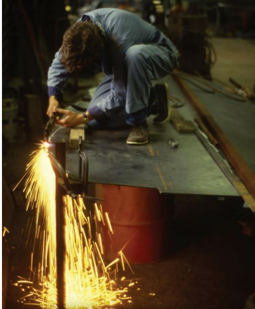
Figure 16. Howard Sutcliffe cutting weathering steel for the Garden Pavilion, 1988. (Photo credit: Shim-Sutcliffe Architects Inc.)
