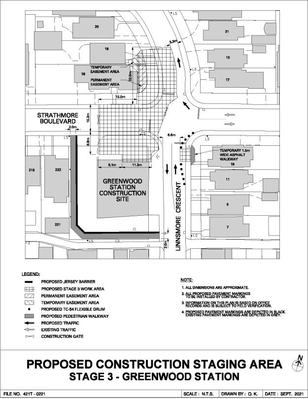
Attachment 2: Proposed Construction Staging Area - Stage 3
