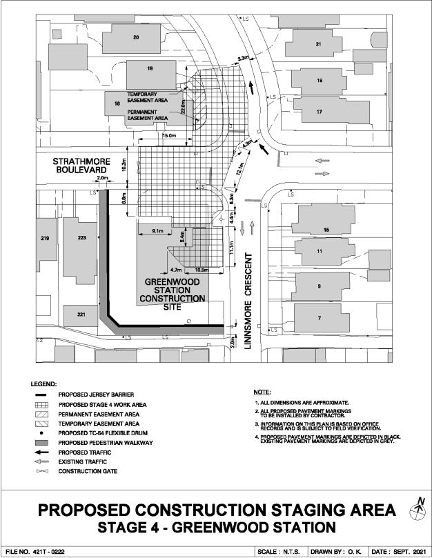
Attachment 3: Proposed Construction Staging Area - Stage 4
