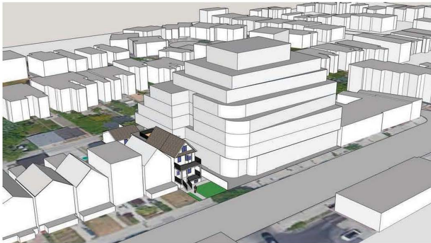
South view of upper storey east and west stepbacks
