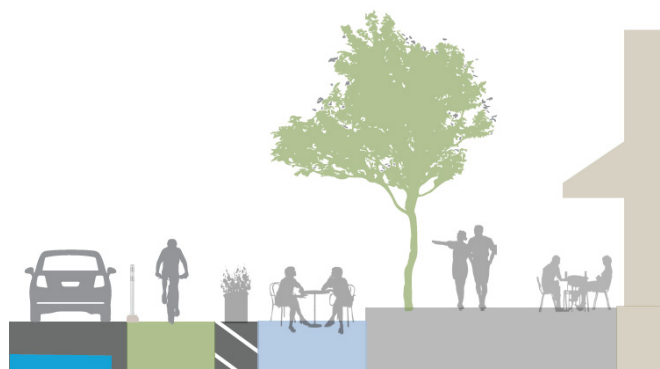
Figure 2: Danforth Avenue Complete Streets Pilot Design Cross Section (with Curbside Patios)
