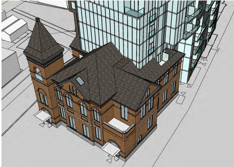
SketchUp model view of 958 Broadview Avenue showing extent of heritage roof (G+C, 2021).
