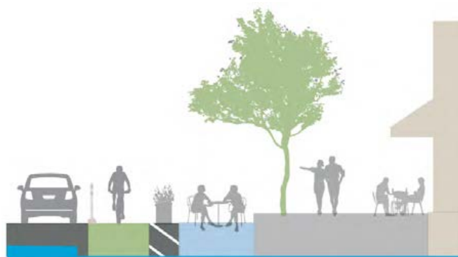
Figure 2: Danforth Avenue Complete Streets Pilot Design Cross Section (with Curbside Patio)
