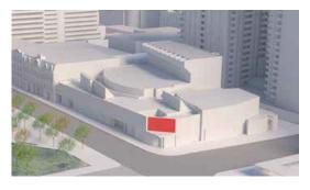
On the west elevation any vertical addition might return closer to the line of the existing west wall while at the same time exposing the original scale and shape of the wall through a setback, reveal in the design.
