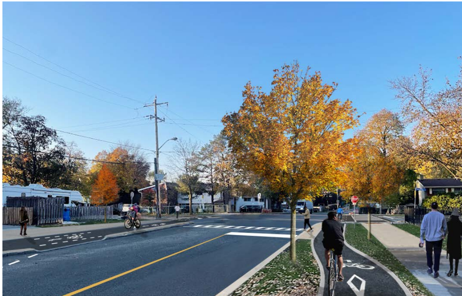
Figure 15: Artist rendering of the proposed design changes on Sentinel Road including raised cycle tracks, new trees and wider sidewalks.
