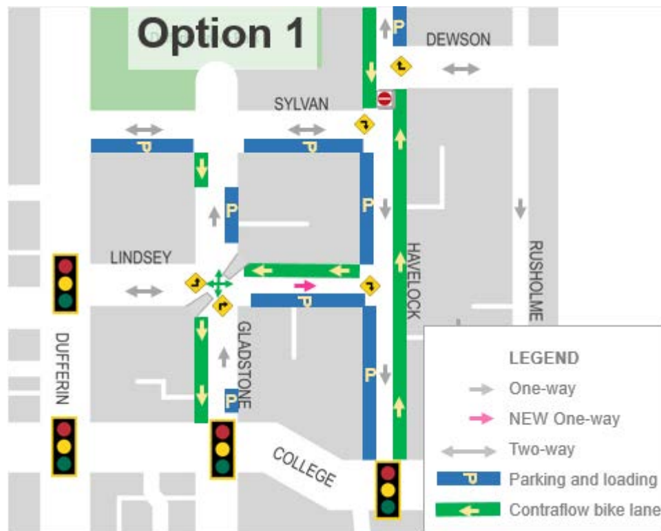
Figure 4: Option 1 on Havelock Street, Lindsey Street, and Gladstone Avenue includes a traffic diverter at Dewson Street and a diagonal diverter at Lindsey Street and Gladstone Avenue.
