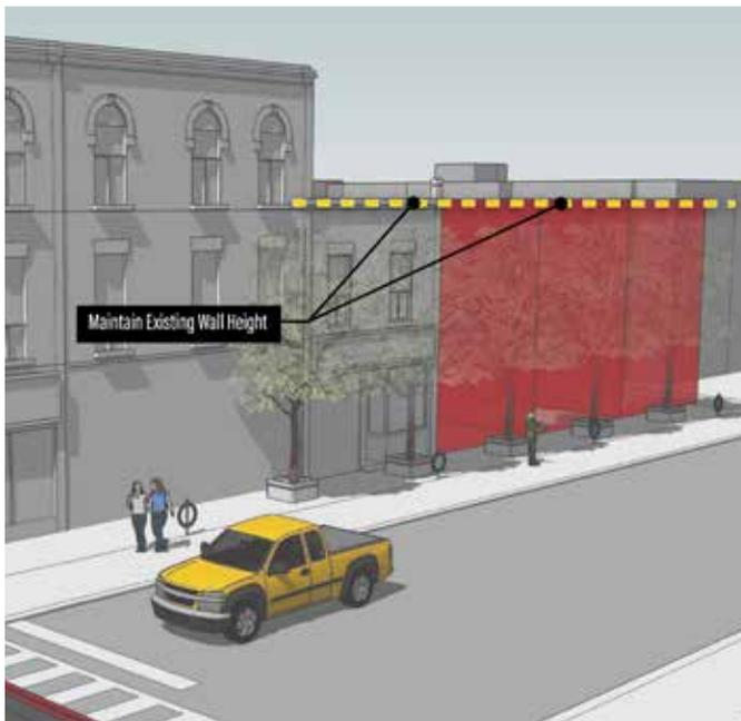
**Figure 71:** *New development on a non-contributing property* shall be designed with a *streetwall* that references the height of *adjacent contributing properties* and *contributing properties* of the block where it is located.
