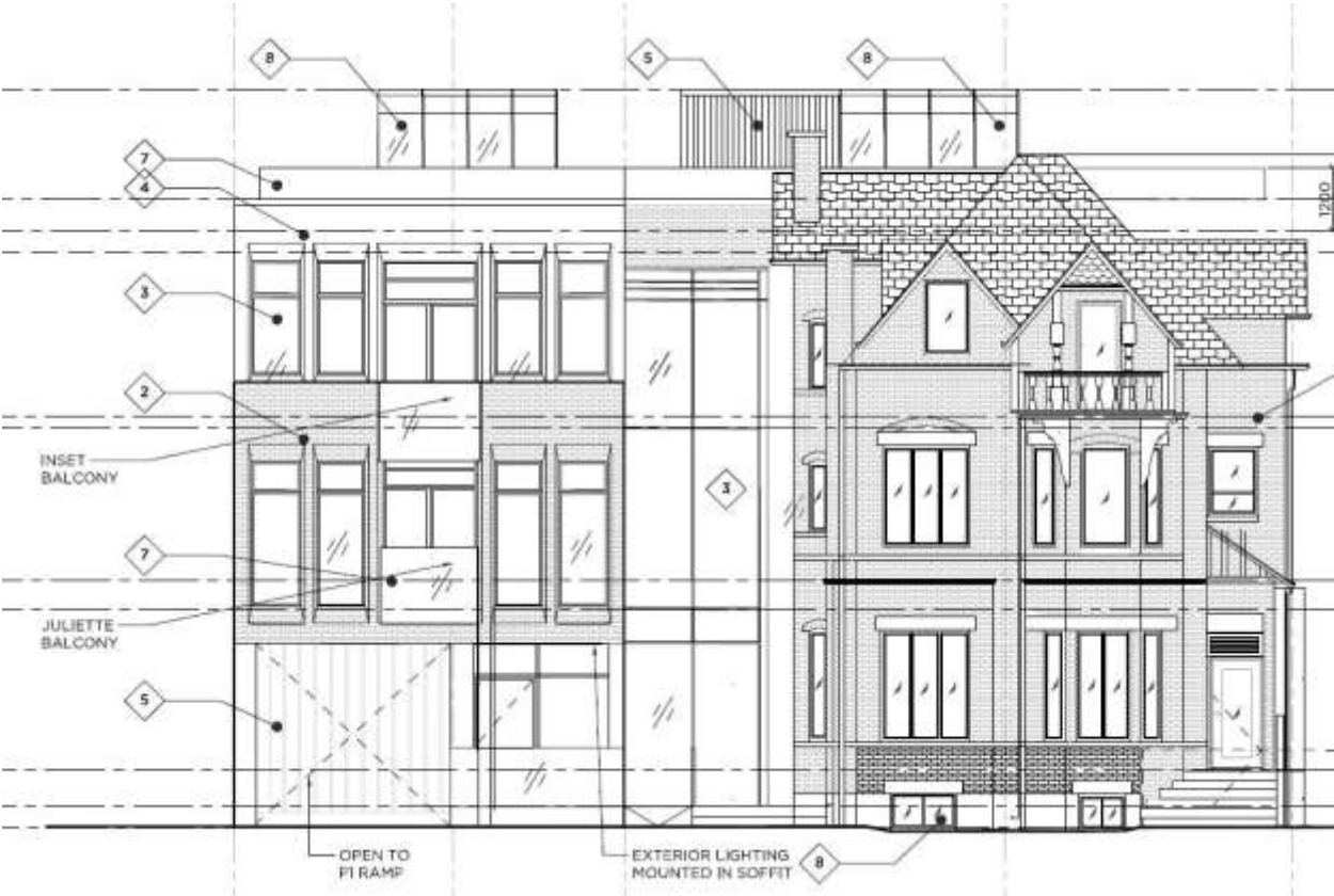
North elevation drawing showing the existing heritage house on the right alongside the new proposal on the left
