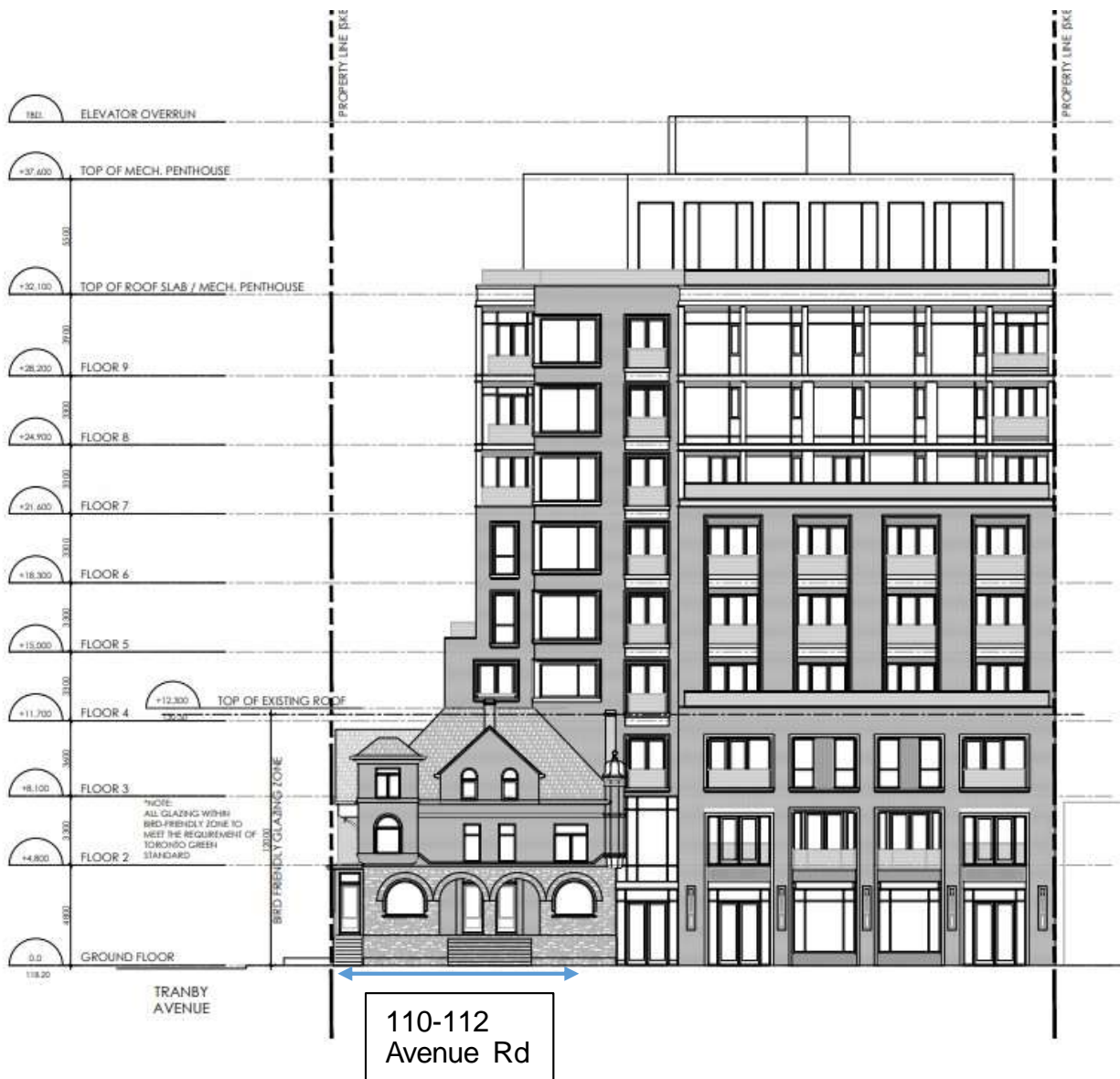
West (primary) elevation facing Avenue Road showing 110-112 Avenue Road to the left, new entry vestibule and new 3-storey townhouse units at base of proposed new building (Richard Wengle Architects, 2022)
