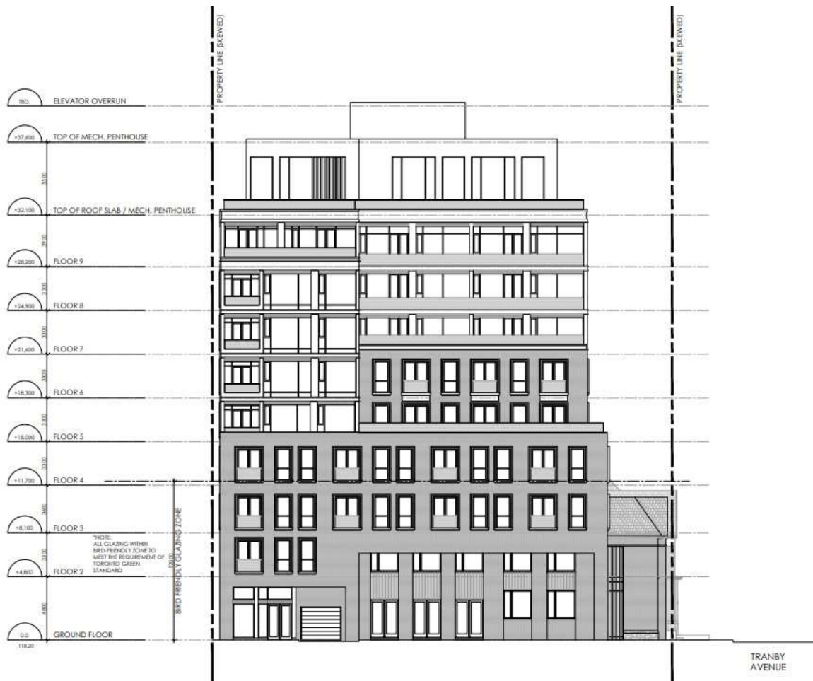
West Elevation-laneway (Richard Wengle Architects May, 2022)
