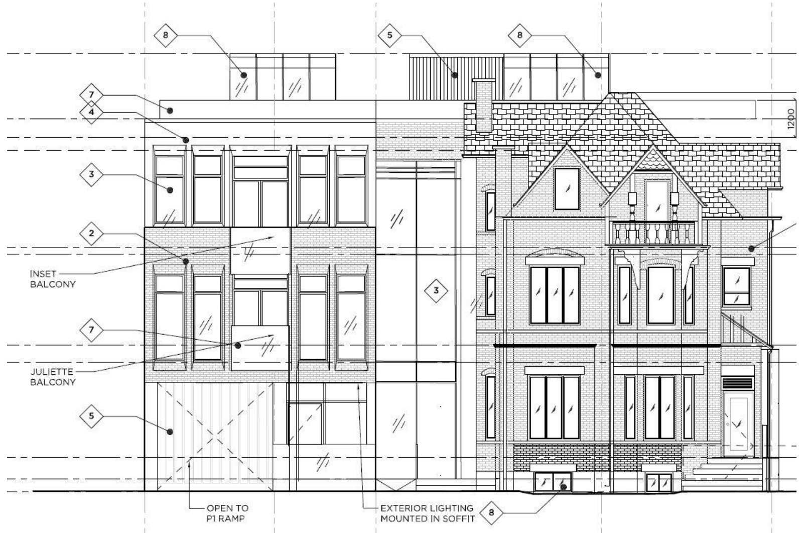
North elevation drawing showing the existing heritage house on the right alongside the new development on the left
