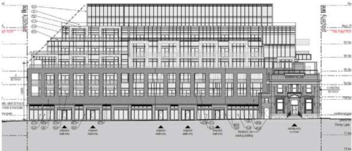
68. Primary (south) elevation of the Development Site (Source: Graziani + Corazza Architects Inc.).
