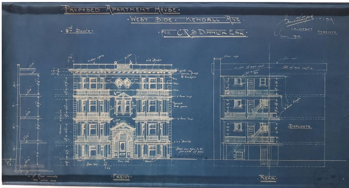
16. Joseph Hunt Stanford's 1912 drawings for a "Proposed Apartment House West Side Kendall Ave" for C.R.S. Dinnick Esq. This image shows the proposed front and rear elevations (CTA).
