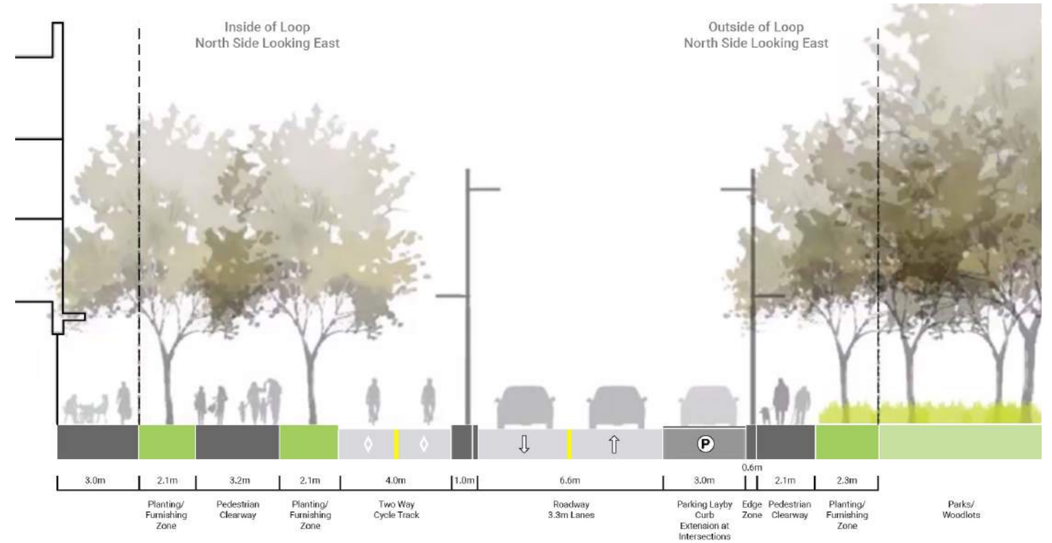
Fig 21. Borough Drive Section
