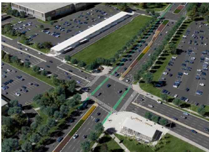
Figure 26: Bus terminal setbacks to preserve a development parcel on the street frontage, Science Centre Station (Photo Credit: Metrolinx)
