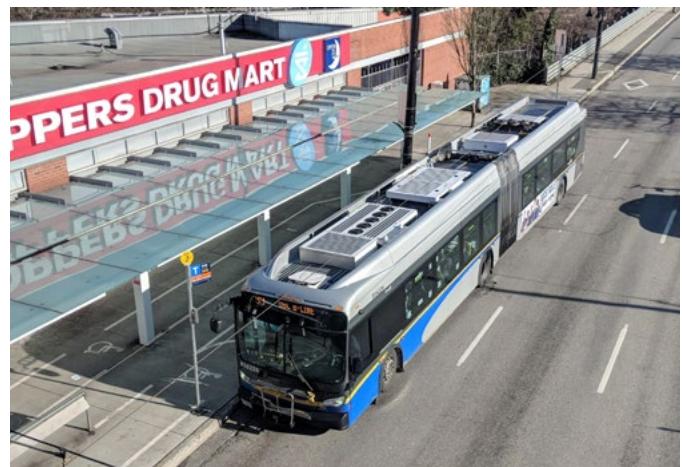
Figure 47: Weather protection integration into adjacent building frontages, clear prioritization of bus space and sidewalk markings to support loading areas - Commercial Broadway Station, Vancouver, BC (Photo Credit: Wiki Commons)
