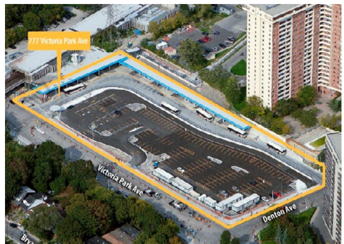
Figure 27: Bus terminal configuration around perimeter of site allowing for future redevelopment of commuter parking at 777 Victoria Park Ave. The yellow boundary denotes entire property, not specific to development site (Photo Credit: CreateTO)
