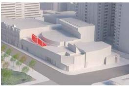
The NW corner was chamfered at 45-degree to include a display feature facing downtown. The new addition should recognize the importance of this corner of the building. Any new feature in the vertical addition should respect the original form of the building and if possible, the original 45-degree feature.
