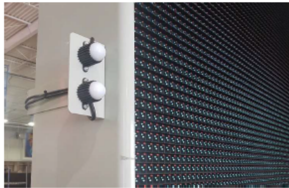
Figure 1. Media Resources standard - dual ambient brightness measuring photocells for hardware redundancy
