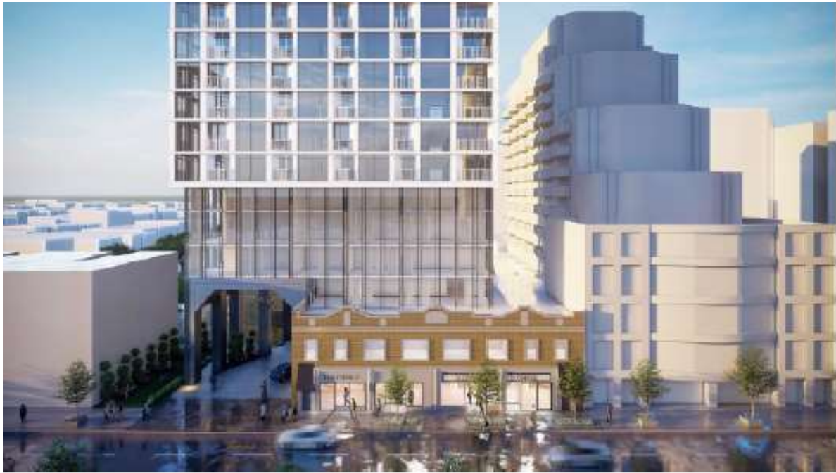
Rendering of project along Yonge Street illustrating the retained buff brick building at 1420 Yonge to the right, entry to the residential units located through a new "vestibule" to the south, and integrated into the base of the tower that is stepped back to allow 1420 Yonge Street to remain as a prominent element along Yonge Street (IBI Group)
