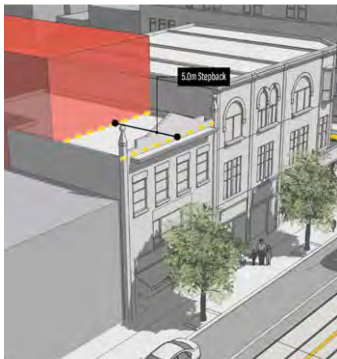
Figure 54: New development and additions above the primary structure of contributing properties shall provide a minimum stepback of 5.0 metres from the streetwall fronting onto Queen Street West.
