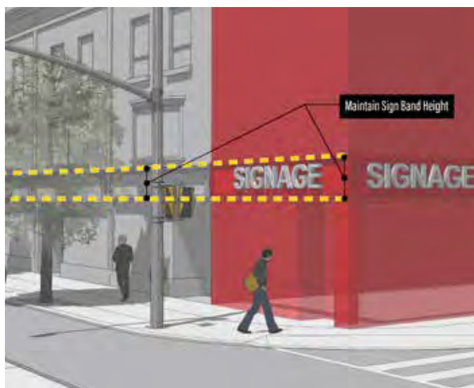
Figure 75: Storefronts should incorporate traditional compositions of storefront components.
