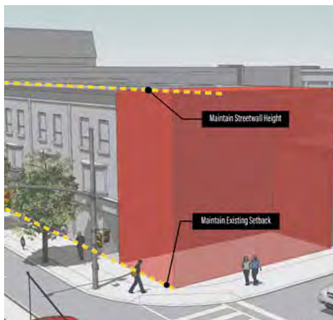
Figure 70: New development on a non-contributing property shall be set back the same distance as the primary structure on adjacent contributing properties and contributing properties of the block where it is located.
