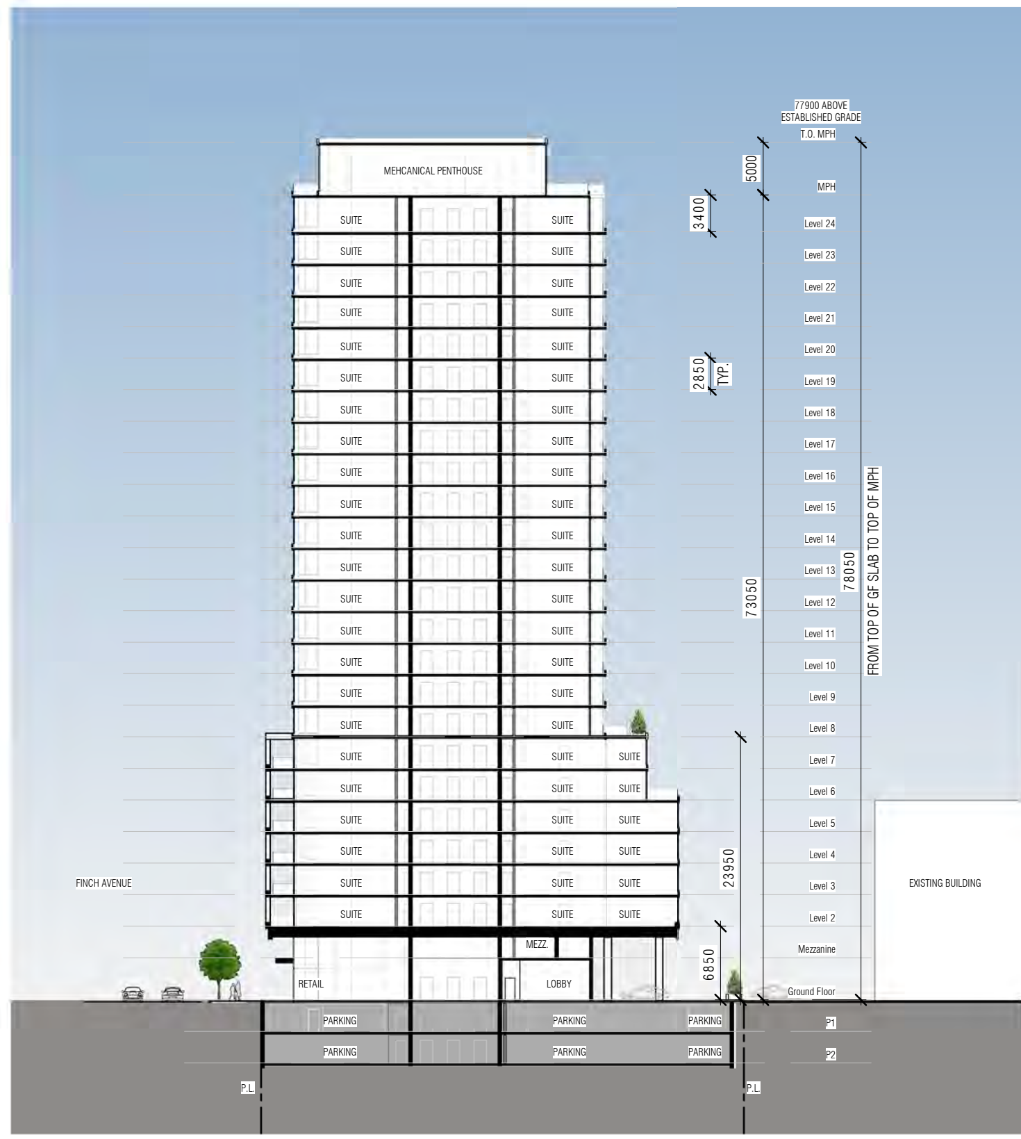
(A) North-South Building Section 1 : 500
