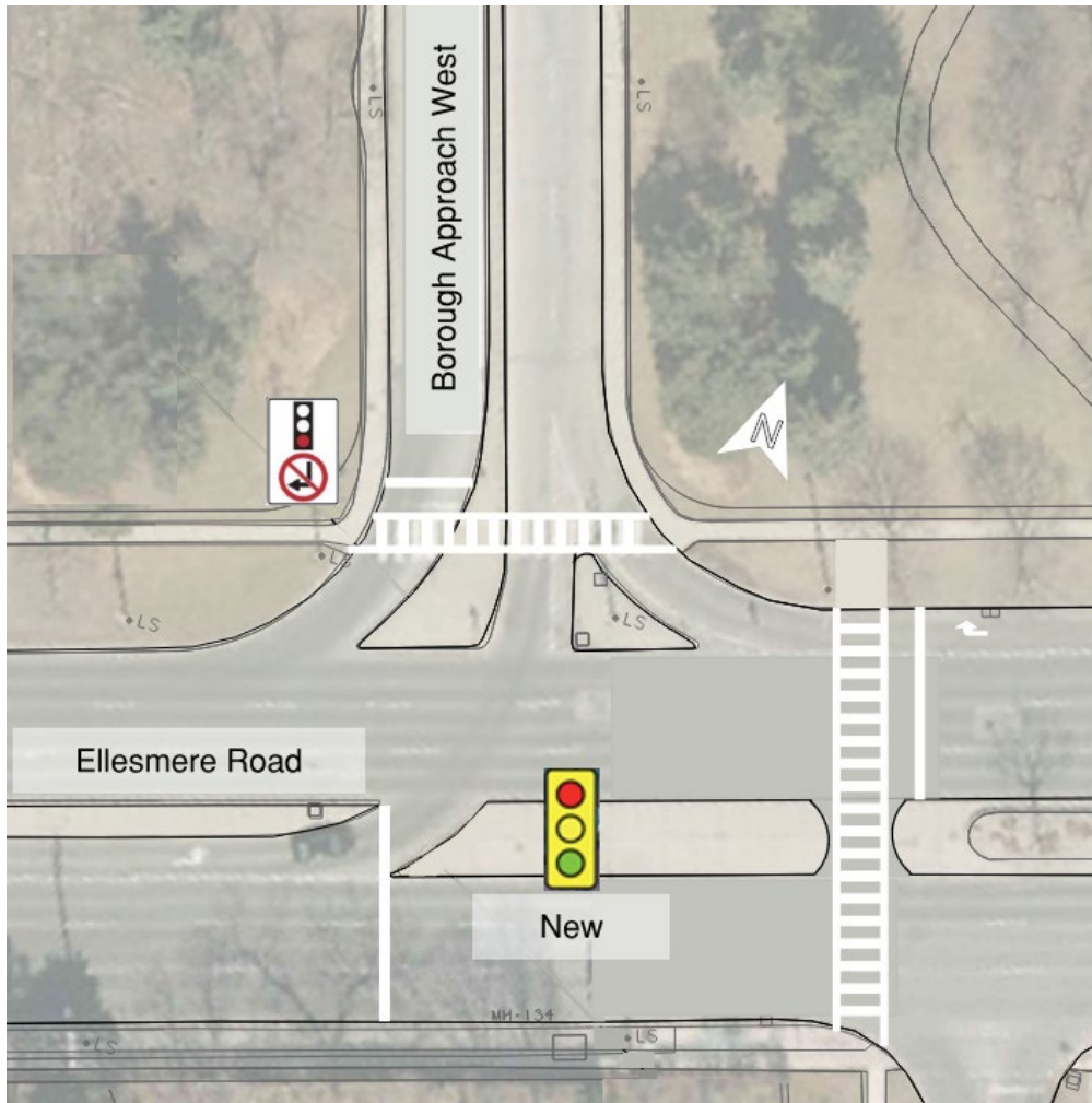
Figure 10. Proposed new traffic control signals at Ellesmere Road and Borough Approach West
