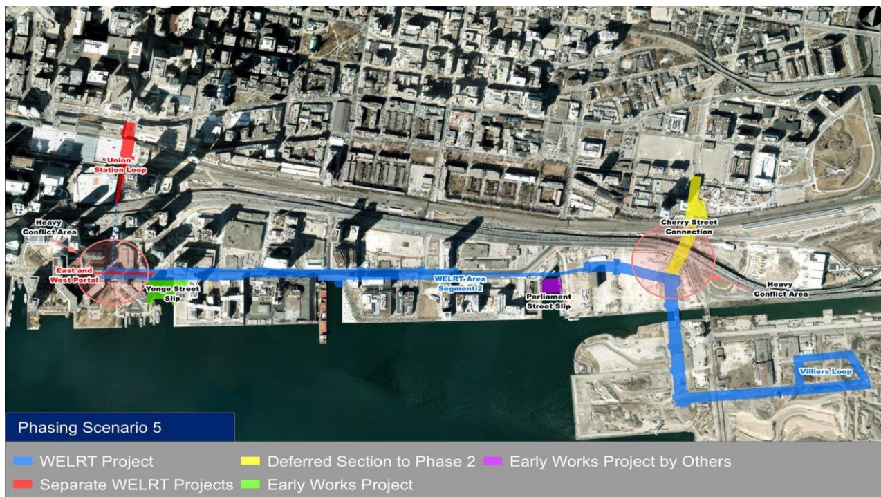
Figure 7 – Scenario 5 - Union Loop, East-West portals and Queens Quay Ferry Docks Station are delivered as a sub-project to maximize underground works specialization. The remainder of the WELRT will be delivered as a sub-project. The Cherry St connection complexity will be addressed by delivering it as a separate phase in the future.
