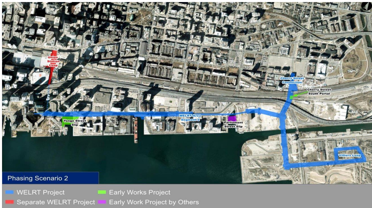
Figure 4 – Scenario 2 - Union Loop as a single sub-project and the remainder of WELRT delivered as a single sub-project. It will increase contractor specialty at Union Station.
