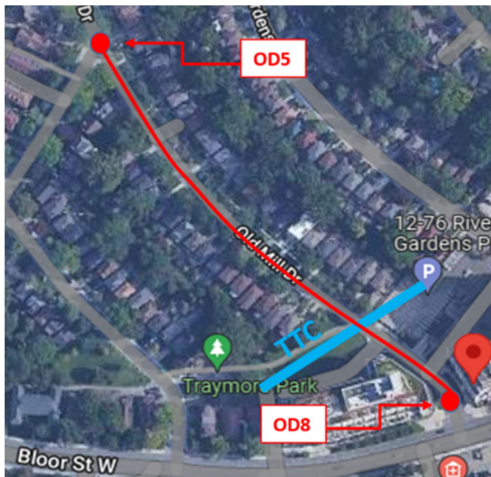
Figure 1: Location of proposed 900mm diameter storm sewer on Old Mill Drive between maintenance holes OD5 and OD8
