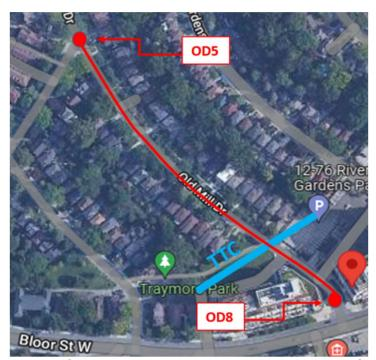
scope of work included crossing Toronto Transit Commission's Line 2 subway tunnel just north of maintenance hole OD8. The Contractor retained a micro-tunnelling subcontractor, Earth Boring CO Limited, to complete the micro-tunnelling work.
