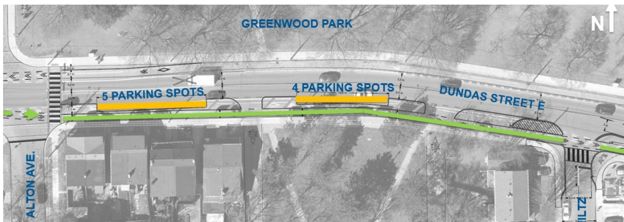
Figure 16: A plan view of the proposed cycle track on the south side of Dundas Street between Alton Avenue and Hiltz Avenue.
