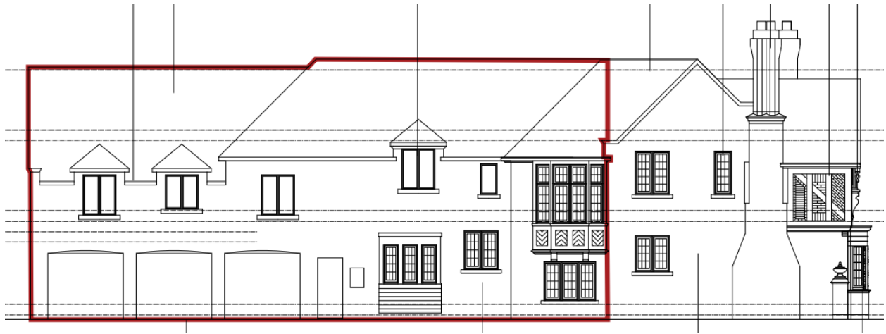
Existing north elevation with red outline area indicating portion of house to be removed. (Source: Wayne Swadron Architects, 2022)
