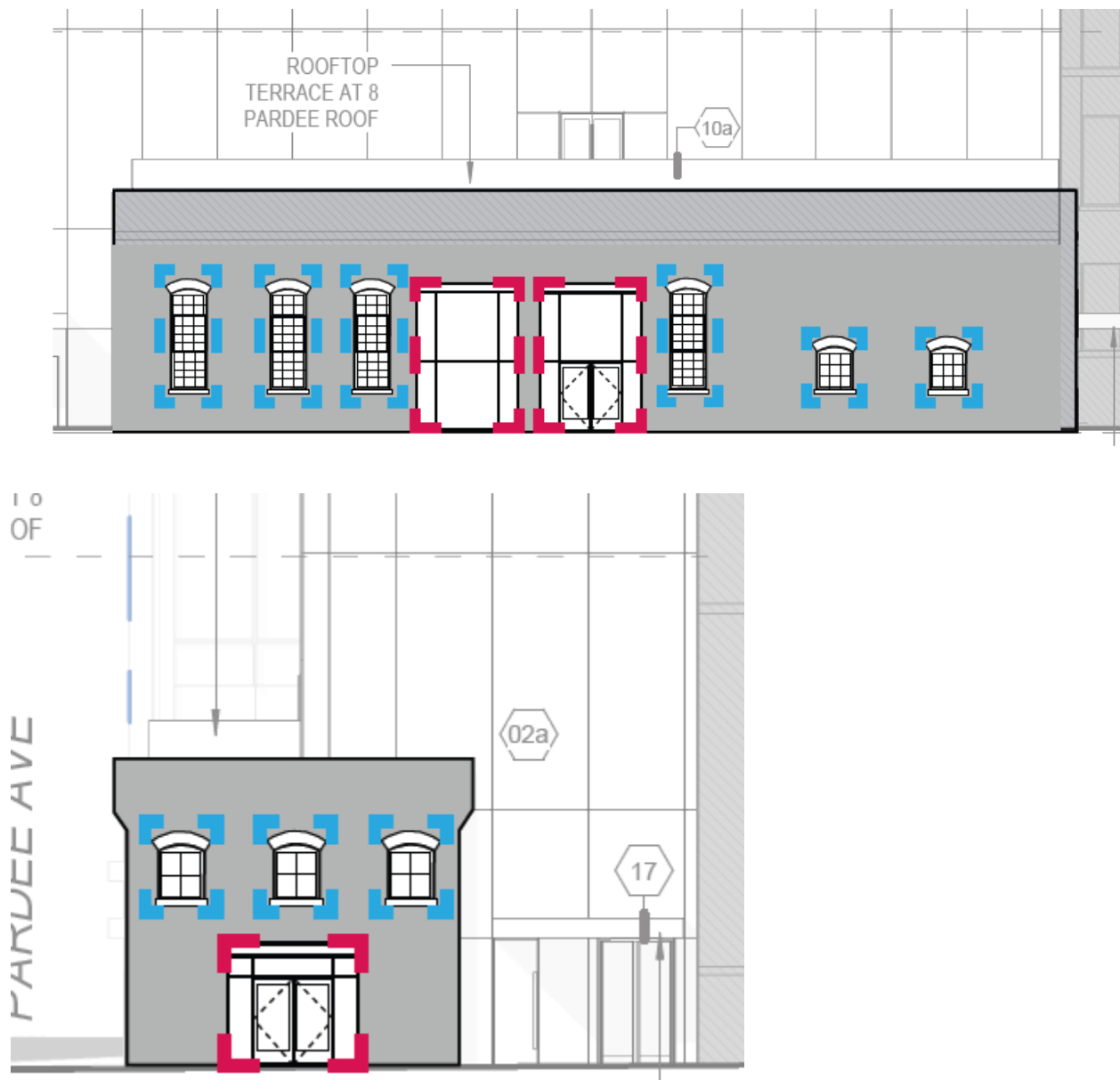
Proposed elevations of reconstructed powerhouse building with reconstructed windows highlighted in blue and new openings highlighted in red. E
