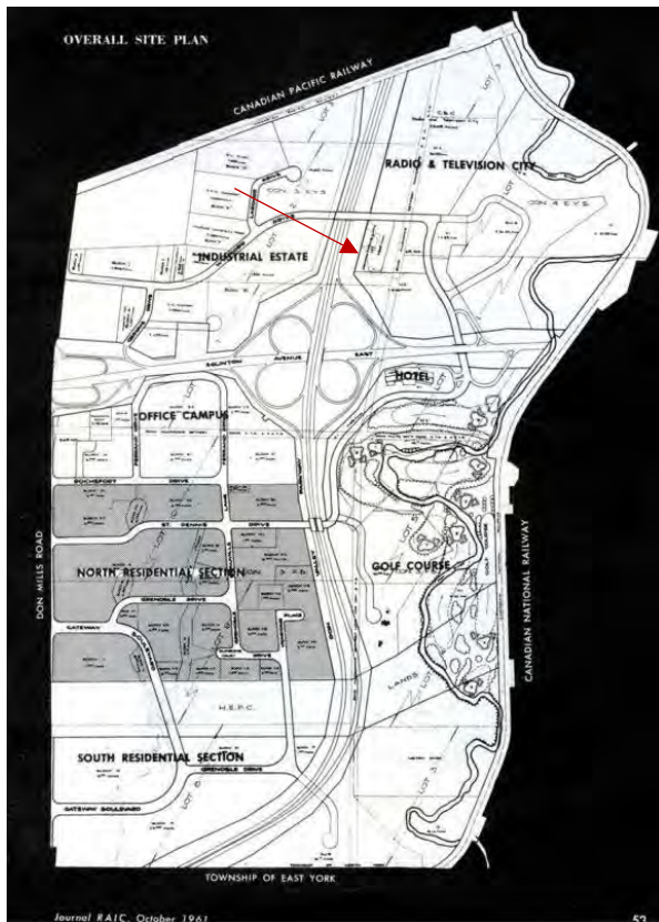
6. Overall Site Plan for Flemingdon Park. The planned community was divided into zones with a high-density residential area taking up about one-third of the entire 500-acre development. Another one-third was for industrial/office/commercial and the final one-third was for green space. The subject site, approximation marked by the red arrow, is situated in the “Radio & Television City” industrial lands portion of the plan (Flemingdon Park, RAIC Journal, October 1961)
