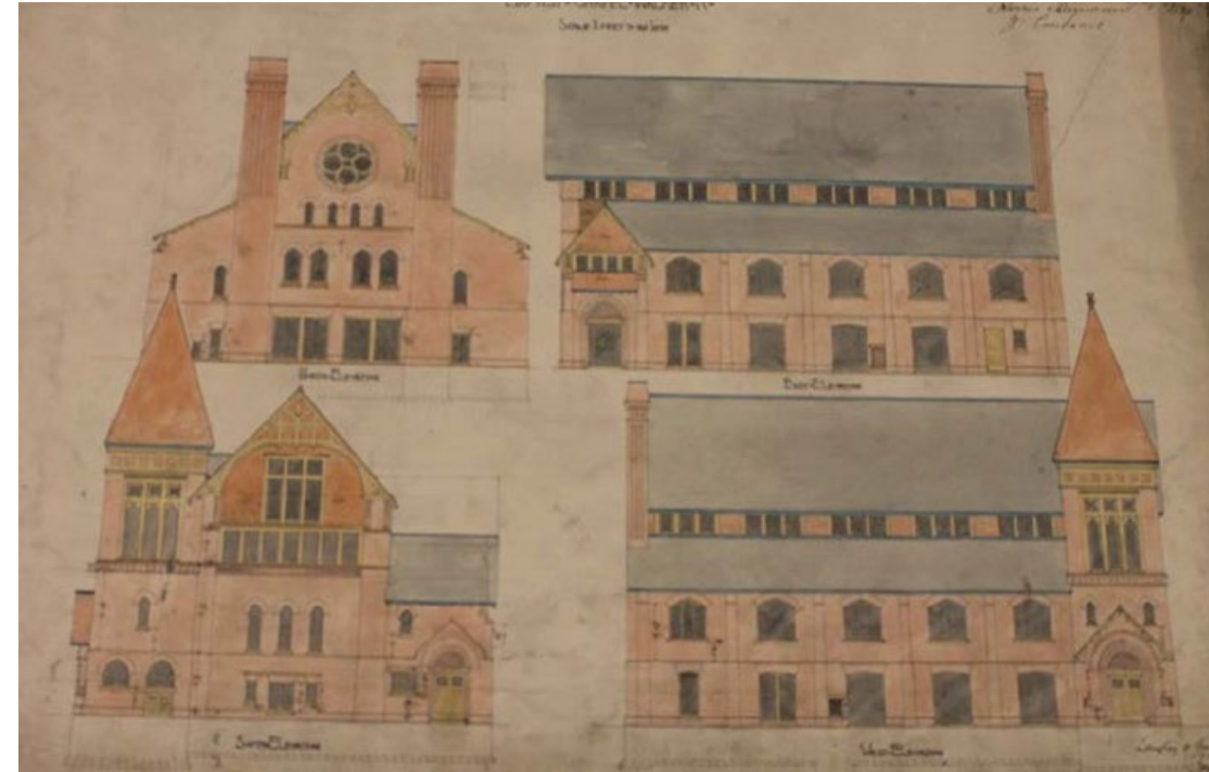
Each elevation of the Sunday School from Langley and Burke's original architectural drawings, 1892. Note: the original form with sides flanking the nave and the original fenestration of the main façade. These plans are the inverse of what was built and likely reflect the design for the originally planned site closer to Walmer Road (Archives of Ontario)
