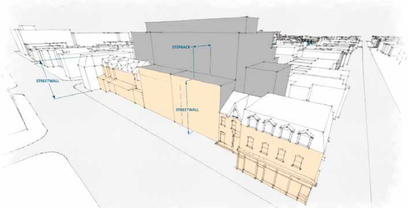
Figure 84: Diagram illustrating new development in the Dundas and Gerrard residential character sub-area that maintains the streetwall height. Its rear portions are higher than the primary structures of neighbouring contributing properties and it has a stepback aligning with the primary structures of neighbouring contributing properties .
