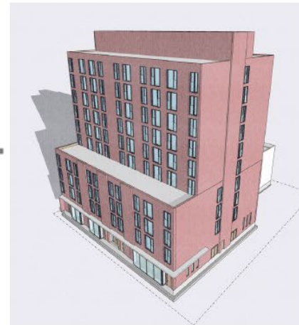
Enclose building with remaining exterior walls and roofs
