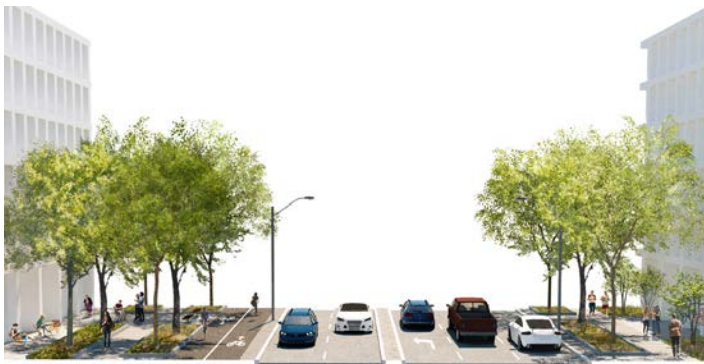
Figure 5.8 Green Loop street design: broad sidewalks, two-way cycle track (where possible), double rows of trees in open planters and other substantial planted areas. More details can be found in the Urban Design Guidelines for streets.
