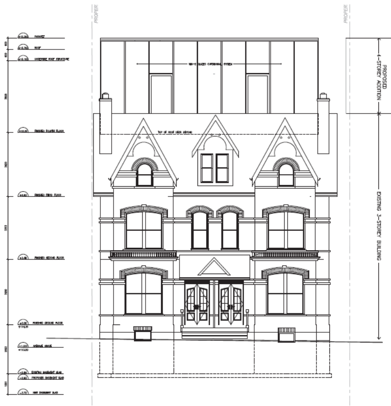
Primary (north) Elevation
