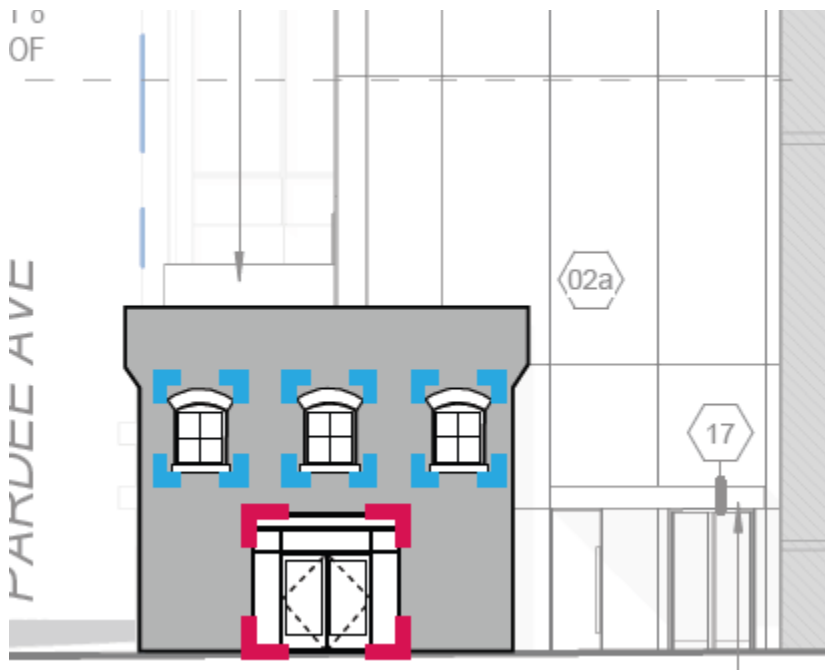
Proposed elevations of reconstructed powerhouse building with reconstructed windows highlighted in blue and new openings highlighted in red. E
