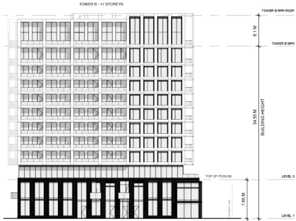
Tower B - North Elevation
