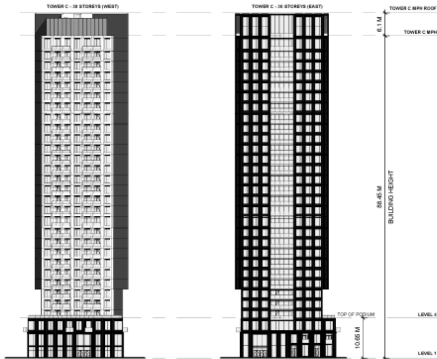
Tower C - West/East Elevation
