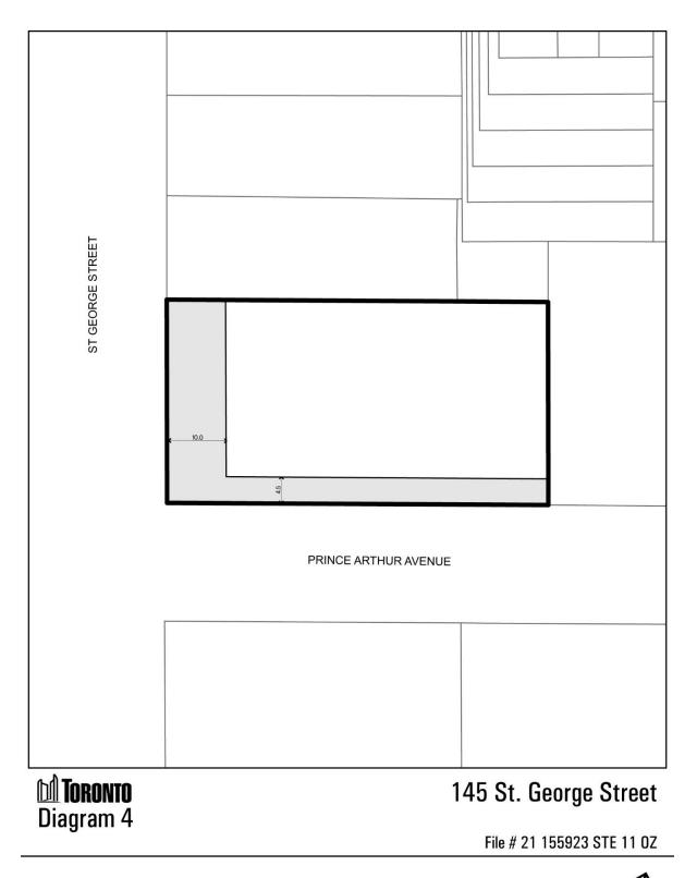
No part of a building, except for any structural elements associated cladding and architectural features, may be located between the Canadian Geodetic Datum elevation of 116.1 metres and a minimum vertical clearance of 4.5 metres in the shaded area.
