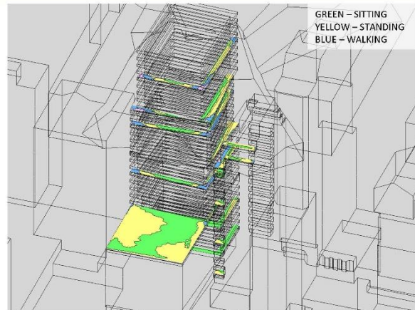
FIGURE 2A: SPRING – NEARBY BALCONY/TERRACE WIND CONDITIONS, NORTHWEST VIEW - EXISTING
