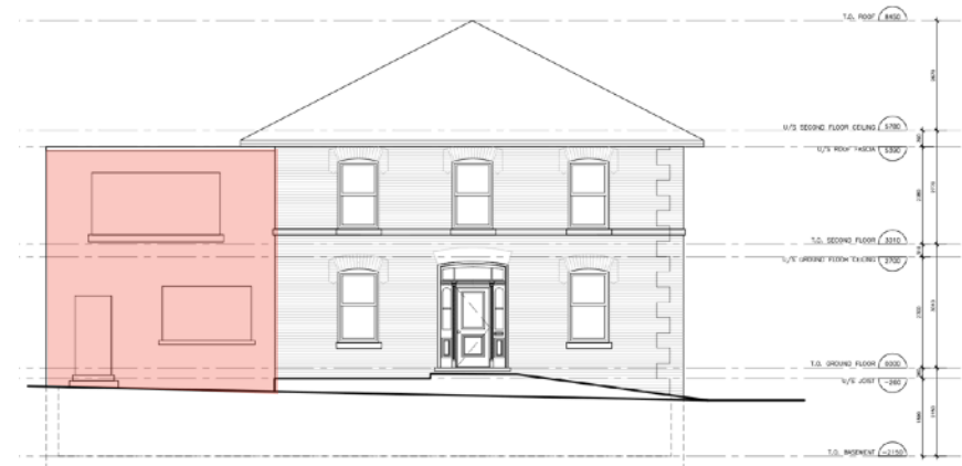
South Elevation: Non-original fabric added the west elevation of the 'Musson House' will be removed. A portion of the eastern elevation will be reconstructed to help
