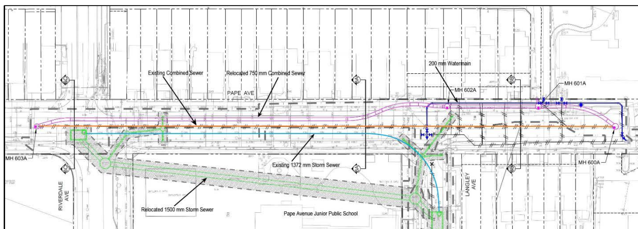
Figure 5 – Pape and Riverdale Advanced Works – Location of New Combined Sewer, Watermain and Storm Sewer
