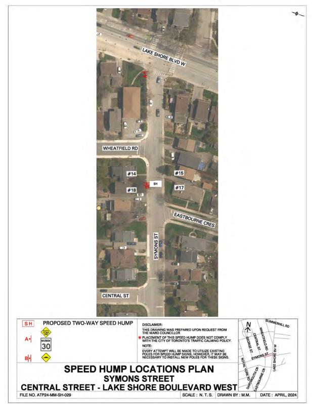
Attachment 31 - ATP24-MM-SH-029- Speed Hump Location Plan
