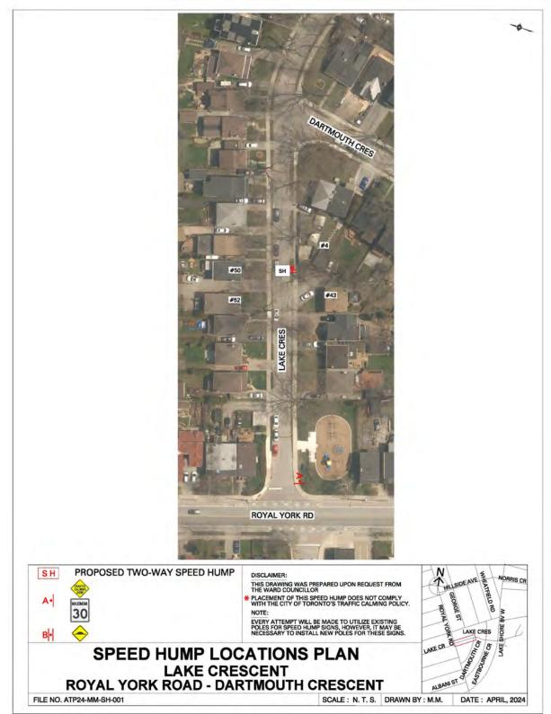
Attachment 3 - ATP24-MM-SH-001- Speed Hump Location Plan
