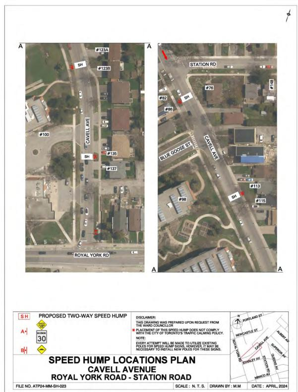
Attachment 26 - ATP24-MM-SH-024- Speed Hump Location Plan
