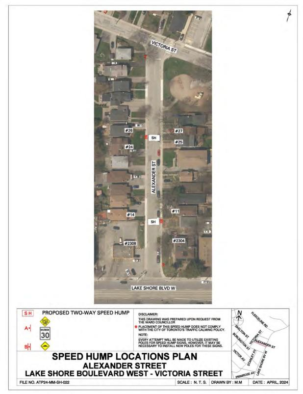
Attachment 24 - ATP24-MM-SH-022- Speed Hump Location Plan
