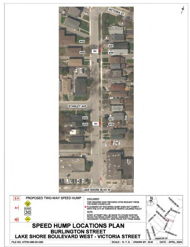
Attachment 22 - ATP24-MM-SH-020- Speed Hump Location Plan
