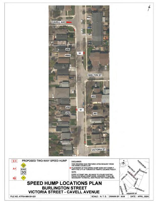
Attachment 23 - ATP24-MM-SH-021- Speed Hump Location Plan
