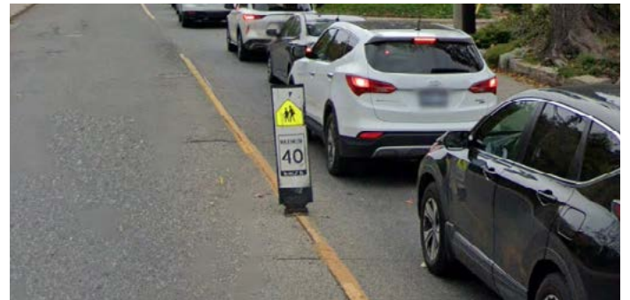
Figure 122. In-road flexible speed signs are installed in the centre of the road, as a visual reminder and a physical device - Oakwood Avenue, Toronto (Google Maps)
