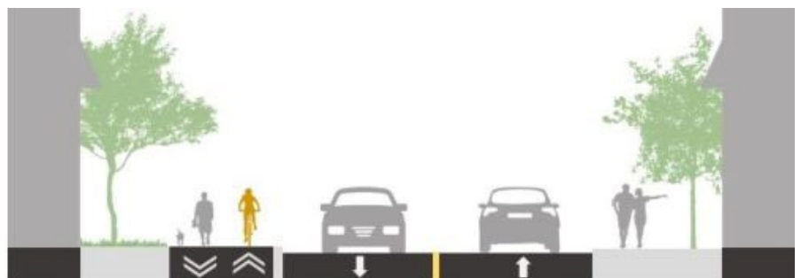
Figure 4: Illustration showing proposed lane and sidewalk changes on Roselawn Avenue and Elm Ridge Drive facing south.
