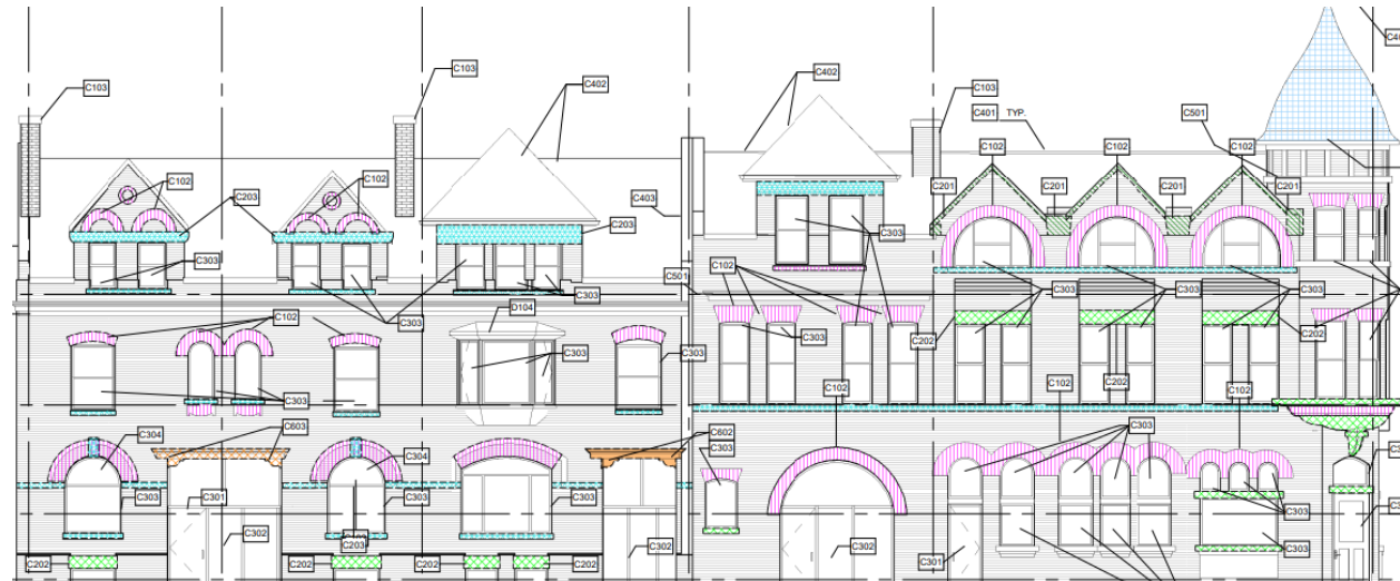
Elevations of reconstructed facades
