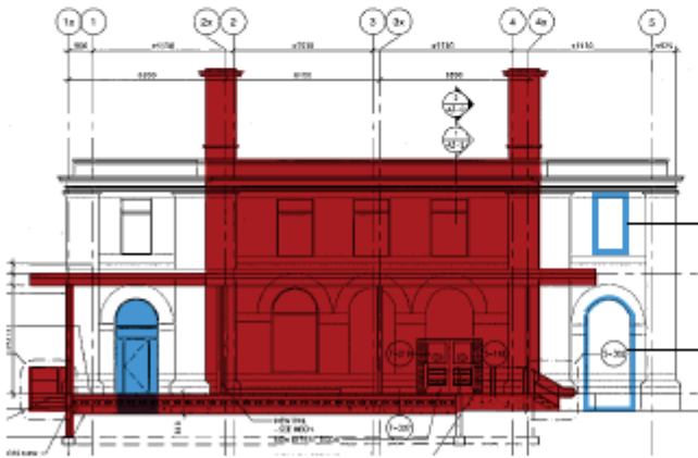
2012 drawings of Postal Station 'C' annotated with proposed alterations, areas of demolition (Canada Post, Annotated by ERA).
