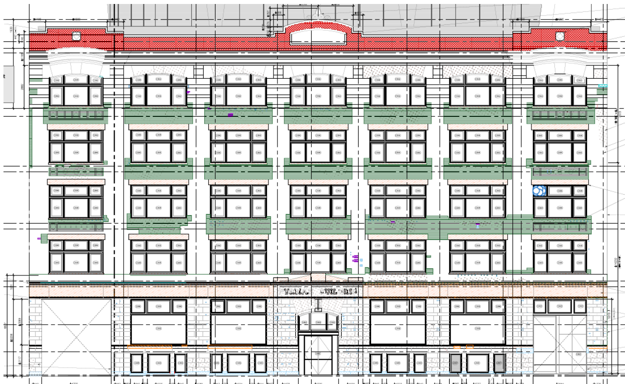
Elevation showing conservation/restoration treatments to front façade (red = rebuild, green = repoint, yellow = new precast or stone units to match original) (Source: ERA Architects Inc.)
