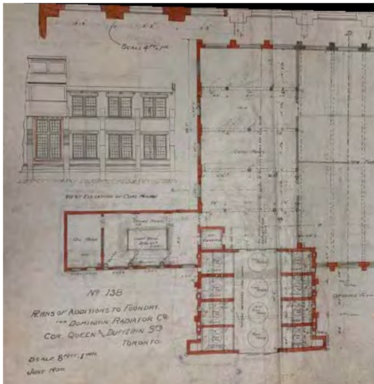
Image 10: 1900 original drawing by EJ Lennox showing a ground floor plan of the Mixing Building, Core Oven Building and south end of the Foundry (right); at top left is the west elevation of the Core Oven Building abutting the south end of the Foundry with its original clerestory and gable roof (EJ Lennox Fonds, Archives of Ontario)
