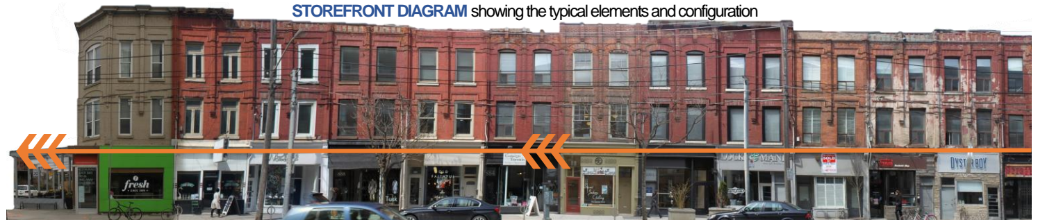
Queen Street West near Crawford Street, c.2017, showing the storefronts at street level whose sign bands create a strong DATUM LINE
