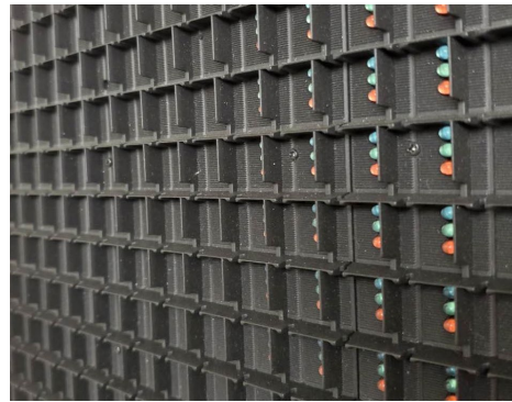
Figures 4 and 5. Close up photographs of SITELINE module face viewed from front (left) and from side (right). Note the red, green and blue diode lenses are directly visible from front direction but are obscured behind baffles viewed from the side.
