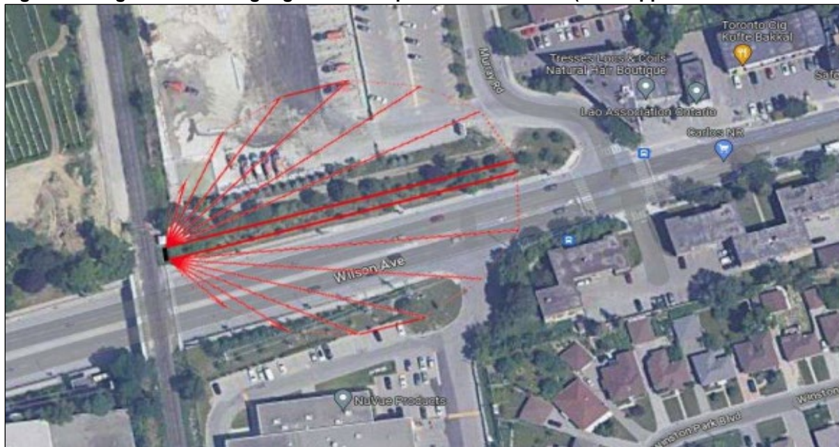
Figure 8: Diagram Illustrating Light Shed Dispersion at 150 NITS (from Applicant's Submissions)
